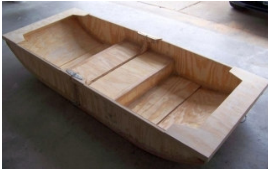
Unfinished Hull Assembled
